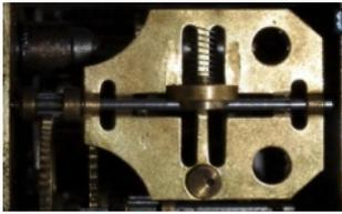
Fig. 2. Mechanism used in clocks in order to stabilize rotational speed – the example of variable moment of inertia  $J$ , dependent on angular velocity  $\omega$
