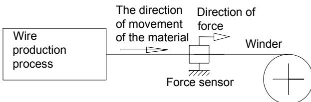
Fig. 1. Location of the sensor in a simplified schematic wire production.
