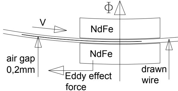
Fig. 5. Details of the scheme of Fig. 4 used for calculation
