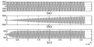
Fig. 5. Output waveforms of class-E power amplifier (a) reference output voltage (b) output voltage without controller (c) output voltage with PI controller
