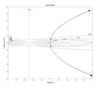
Fig. 9. Nyquist diagram on magnitude and phase margin of PID controller.
