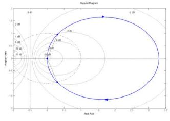
Fig. 10. Nyquist diagram on magnitude and phase margin of VCO controller.
