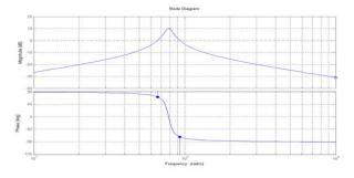
Fig. 8. Bode plot on magnitude and phase margin of VCO controller.
