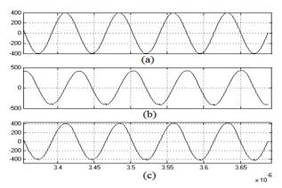
Fig. 6. Output waveforms of class-E power amplifier (a) reference output voltage (b) output voltage without controller (c) output voltage with VCO
