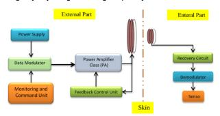
Fig. 1. Biomedical power amplifier with feedback control system.
