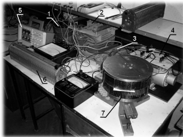
Fig. 4. The experimental setting for research of one phase of rotary transformer: 1 – autotransformer, 2 – transformer, 3 – diode bridge, 4 – synchronous generator with driving DC motor, 5 – digital oscillograph, 6 – load resistor, 7 – rotary transformer
