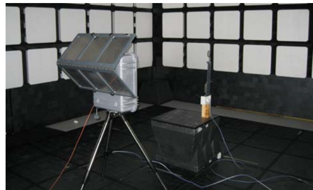
Fig.7. Measuring position for measuring shielding effectiveness with the use of high power generator (arrangement of measuring position during standardization measurement)
