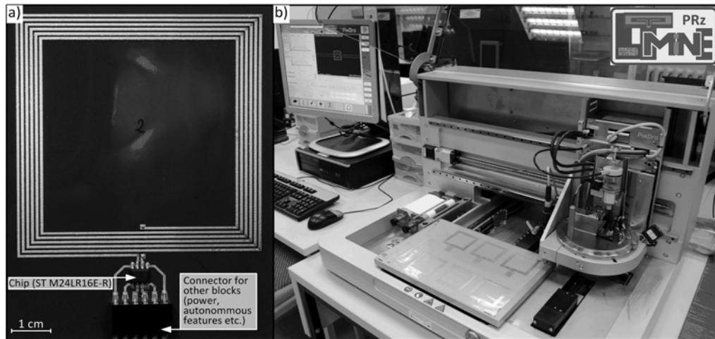
Fig.2. HF RFID semi-passive transponder: a) sample, b) ink-jet printing stand in the author's HYBRID laboratory
