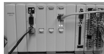
Fig.9. The CECX modular control system consisting of CPU and I/O modules
