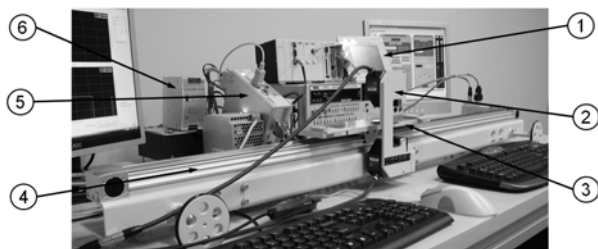
Fig.2. Deformation General view of the Plate Edge Scanner (PES): 1 – control panel, 2 – laser heads, 3 – moving table, 4 – transportation linear module with stepper motor, 5 – PLC controller, 6 - power supply unit
