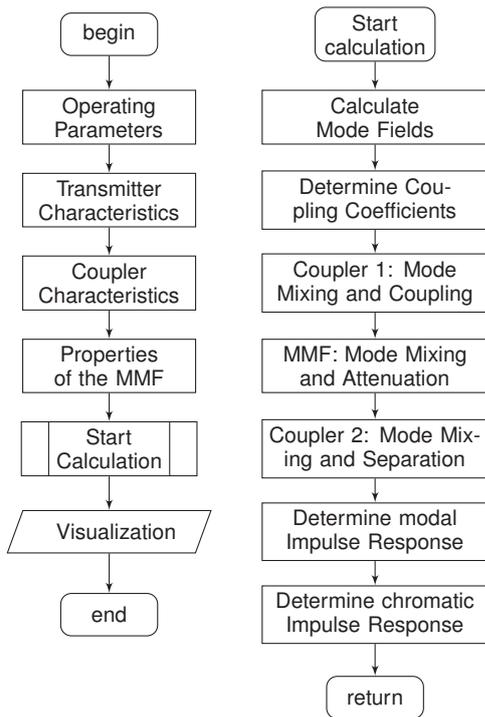
Fig. 3. Flowchart of the simulation
