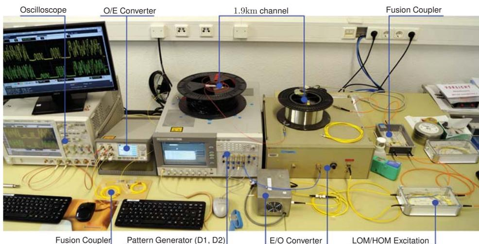
Fig. 1. Testbed for optical MIMO transmission
