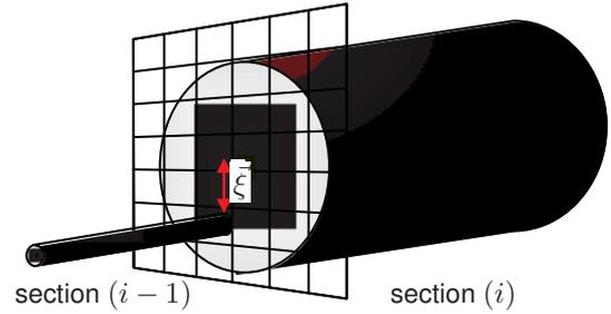
Fig. 4. Principle of mode excitation using a SMF to MMF splice
