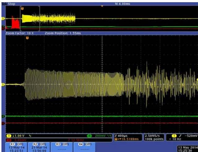
Fig. 2. Waveform of the sample PRIME frame with zoomed preamble and fragment of the header
