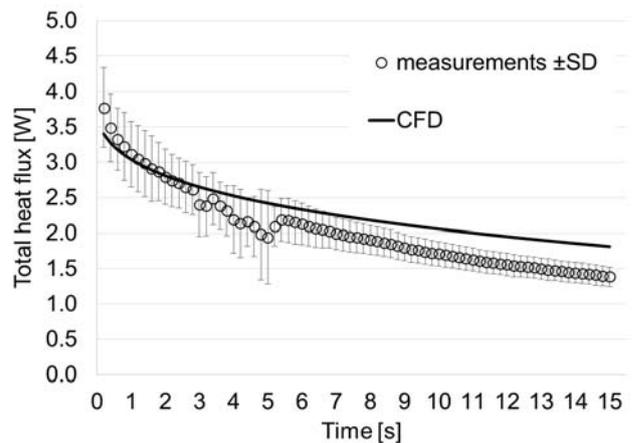
Fig. 10. Total heat flux on compress/skin interface vs. time for experiment (mean  $\pm$ SD, N=8 samples) and CFD simulation
