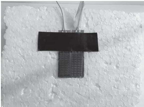
Fig. 6. Measurement setup - brass compress (not visible) located below heat sensors attached to the block of expanded polystyrene (heat insulation)
