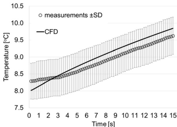
Fig. 9. Compress center midplane temperature vs. time for experiment (mean  $\pm$ SD, N=8 samples) and CFD simulation
