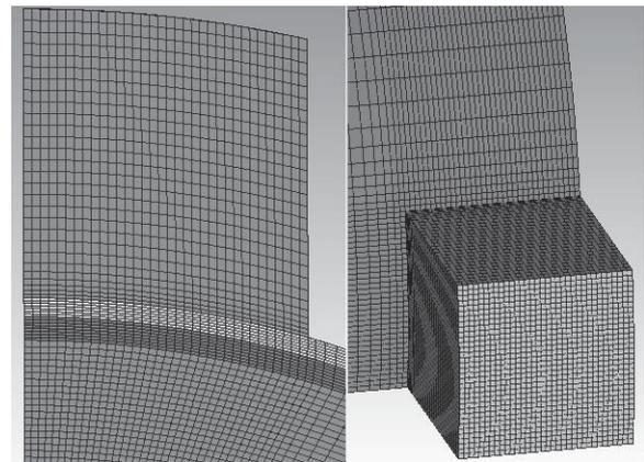
Fig. 4. Selected regions of numerical mesh: in symmetry plane (left) and seen from above the compress (right)
