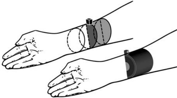
Fig. 2. Scope of modelled region (200mm long section of human forearm), due to symmetry only 1/4 of forearm geometry (gray) and compress (black) is considered (upper sketch). 3-D geometrical model of computational domain representing section of human forearm (lower sketch)
