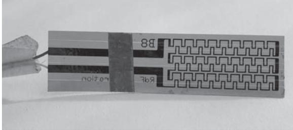
Fig. 5. Micro-Fiol® heat flux sensor (RdF Corp., USA)
