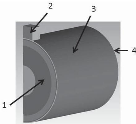
Fig. 3. 3-D geometrical model of computational domain (1 – tissues layers: bone, muscle, fat, inner skin, outer skin, 2 – cooling compress, 3 – forearm outer skin 4 – isolated wall, i.e back & front)
