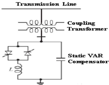
Fig.1. SVC connected to a transmission line
