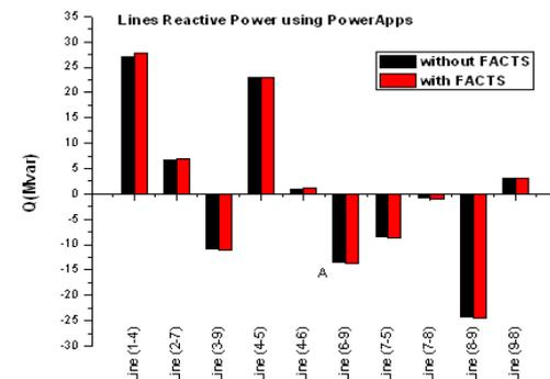
Fig.7. Lines Reactive Power with PowerApps
