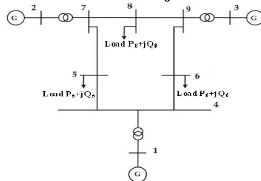
Fig.2. Synoptic scheme of System IEEE, 9 Bus
