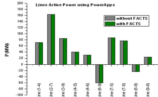
Fig.5. Lines Active Power with PowerApps
