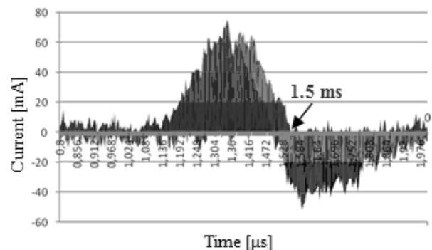
Fig.11. Current waveform during the fuel pressure drop
