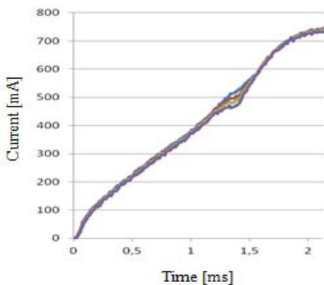
Fig.9. Differences in current characteristics for the same type of the injectors
