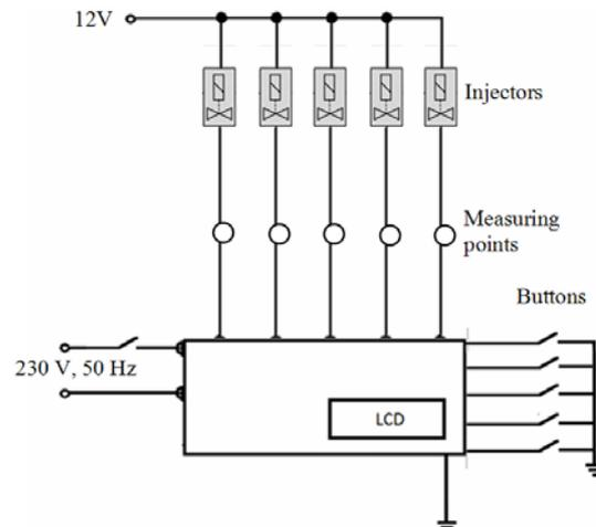
Fig.2. Block diagram of the measuring system
