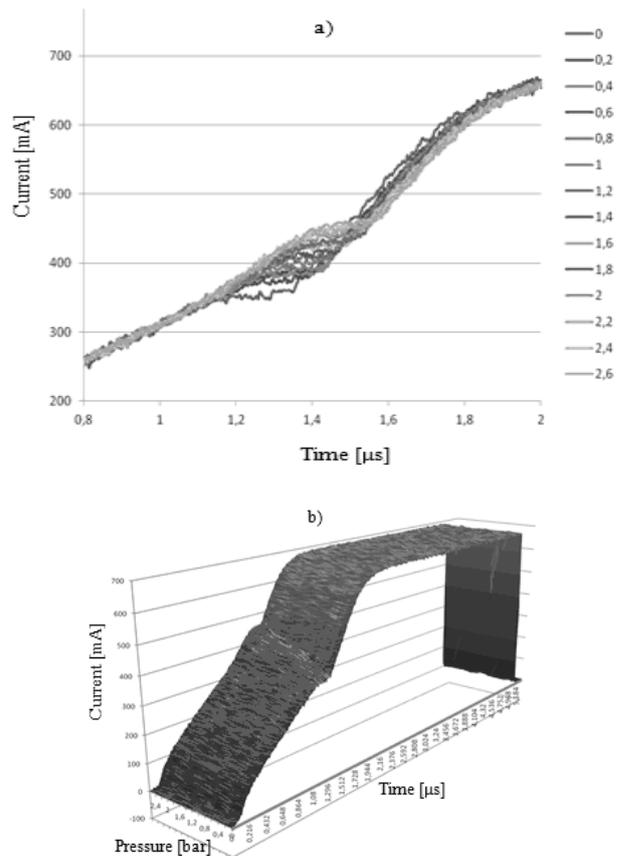
Fig.10. Effect of fuel pressure changes on the current characteristics: a) 2d chart, b) 3d chart
