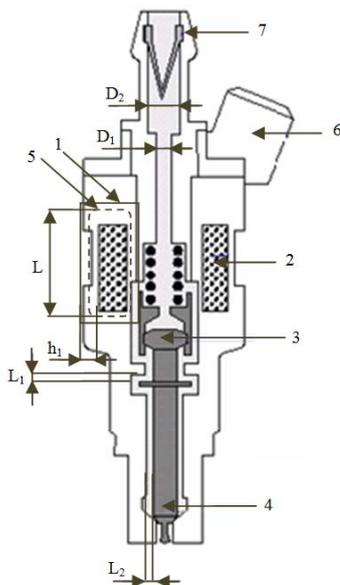
Fig.1. Construction of an electronic fuel injector [4]: 1 – Iron core, 2 – electromagnetic coil, 3 – armature, 4 – needle valve, 5 – yoke of magnet, 6 – electrical connection, 7 – filter
