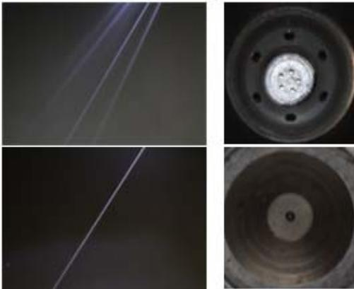
Fig.8. Differences in the injection for different types of injectors
