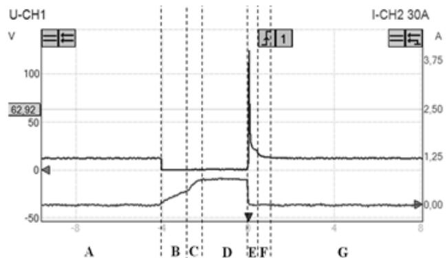
Fig.4. Fuel injector voltage and current characteristics
