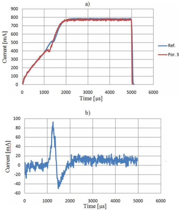
Fig.7. Reference injector current and current at a fuel zero pressure: a) referent and failure currents, b) their difference
