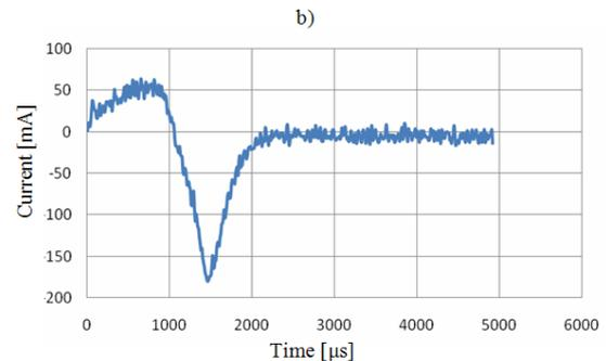
Fig.5. Reference injector current and the current at standstill needle valve in the open position: a) referent and failure currents, b) their difference
