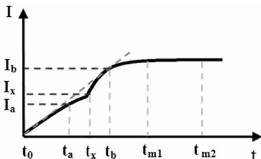
Fig.12. Current characteristic with marked moments of time in which the current measurement allows to determine the state of the injector system
