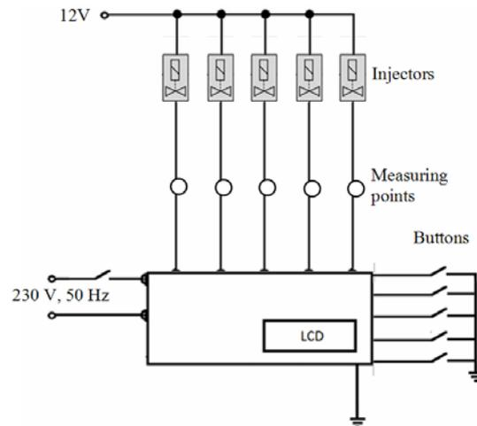
Fig.2. Block diagram of the measuring system
