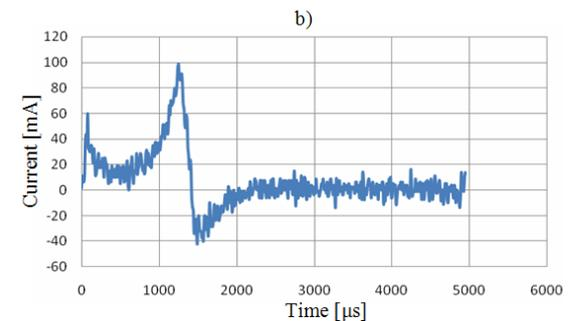
Fig.6. Reference injector current and the partial movement current of the needle valve: a) referent and failure currents, b) their difference
