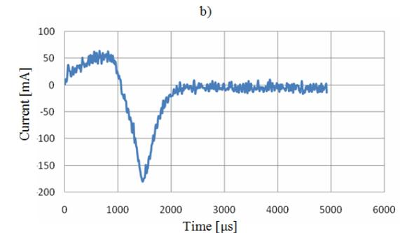
Fig.5. Reference injector current and the current at standstill needle valve in the open position: a) referent and failure currents, b) their difference
