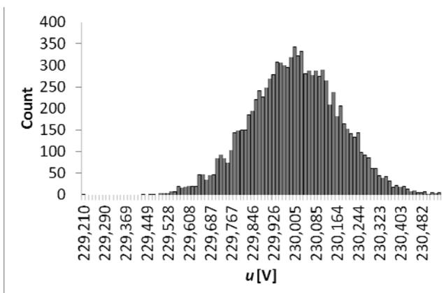
Fig. 6. Histogram for:  $u = 230.0 V$ ,  $k_u = 0.02 V/V$ ,  $f = 500 Hz$
