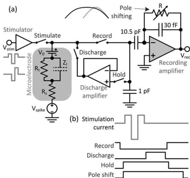
Fig.3. Proposed circuit for artifact minimization: (a) schematic of the circuit, (b) control signals.  $V_{spike}$  represents the neuron activity
