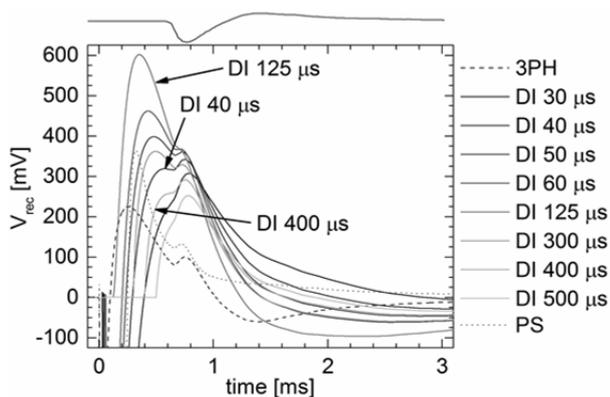
Fig.6. Simulation results: the comparison of responses of neuron cell recorded by the amplifier for three methods of artifact reduction (3PH – triphasic stimulus pulse, DI – discharging the electrode for a given period, PS – pole shifting). In all cases the cell response started 600  $\mu$ s after the end of stimulation (its peak value occurred about 200  $\mu$ s later). The shape of response signal is shown above the top axis
