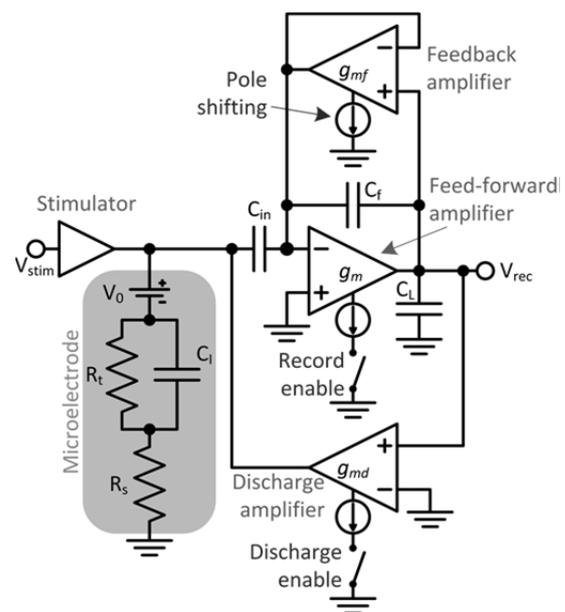
Fig.1. Schematic of fast artifact recovery circuit proposed by Blum, Brown *et al.*: electrode discharging in feedback loop and pole shifting methods are implemented
