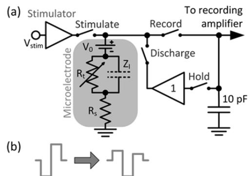
Fig.2. Schematic of fast artifact recovery circuit proposed by Hottowy *et al.*: (a) electrode discharging using sample-and-hold technique, (b) utilization of triphasic stimulus pulse instead of the biphasic one
