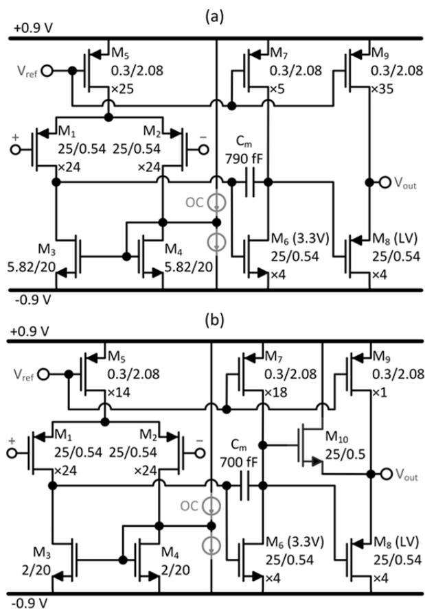
Fig.4. Schematics of: (a) recording amplifier, (b) discharge amplifier. All dimensions are given in  $\mu$ m. OC represents the offset correction circuit
