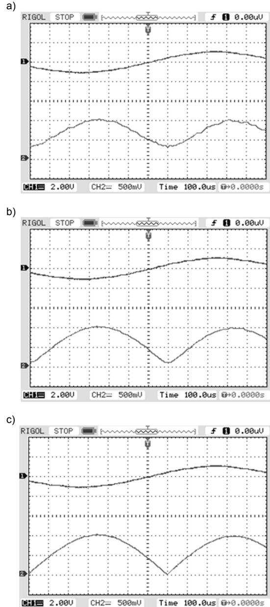
Fig. 7. Input signal  $x(t)$  - 1 and the CAAV characteristic - 2 for  $B_1 = 25\text{ kHz}$  and  $M = 256$ ; a)  $\sigma_1 = 0.45\text{ V}$ ; b)  $\sigma_1 = 0.14\text{ V}$ ; c)  $\sigma_1 = 0.04\text{ V}$
