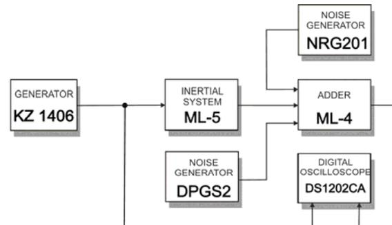
Fig.3. The block diagram of measuring stand
