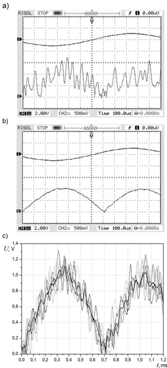
Fig.6. Behaviours of signals: input signal  $x(t)$  - 1 and the delayed signal - 2; a) delayed signal disturbed by noise  $N_1(0, 0.14)$ ;  $B_1 = 25\text{ kHz}$ ; b) delayed signal disturbed by a noise on the level of -30 dB; c) examples of implementation of delayed signals disturbed by a noise on the level of -10 dB and the average value of the implementation (marked in black)
