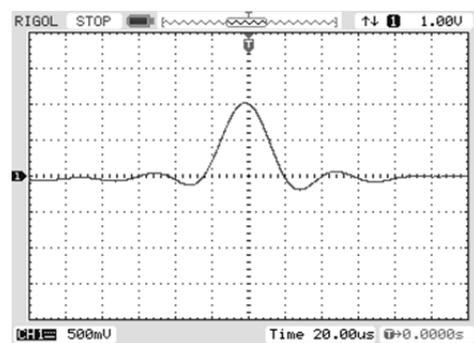
Fig.4. Normalised autocorrelation function  $\rho_1(\tau)$  of white noise in the band  $B_1 = 25$  kHz
