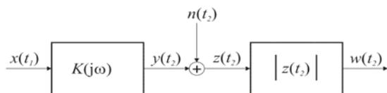
Fig.1. Model of measurement signal processing
