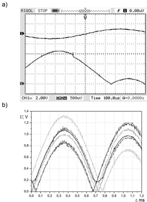
Fig.8. Behaviours of signals  $x(t)$  - 1 and the delayed signal  $y(t)$  - 2; a) delayed signal disturbed by noise  $N_2(0, 0.5)$ ;  $B_2=55$  Hz; b) examples of implementation of delayed signals disturbed by a noise on the level of -10 dB and the average value of the implementation (marked in black)
