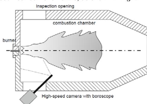
Fig.2. Combustion chamber with camera mounting
