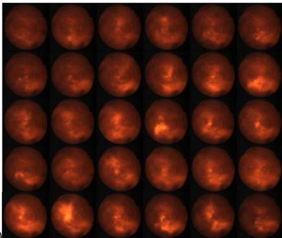
b) Fig.1. The first 30 frames of combustion image sequences: a) stable combustion, b) unstable combustion
