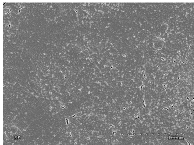
Fig. 1. The SEM image of thin metal layer created on the surface of composite in the PVD process, the magnification 400x, (the surface is made of nylon threads with poliuretan cover - Cordura)
