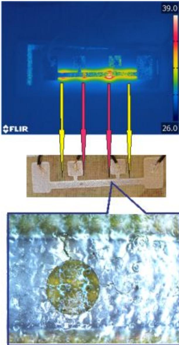
Fig.3. The layer with defect done with laser
