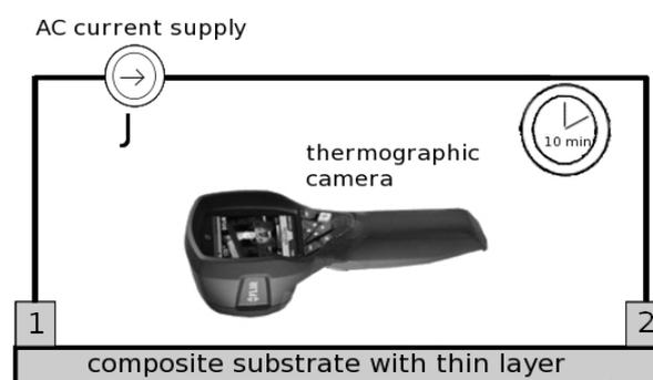
Fig. 2. The stand for taking the thermographic images of thin metal layer - the part of working textronic system
