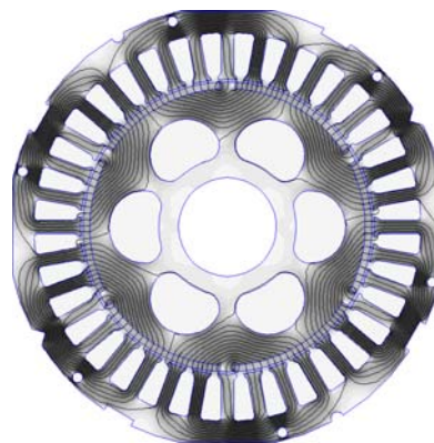
(b) Surface Inset (SI) Magnets
