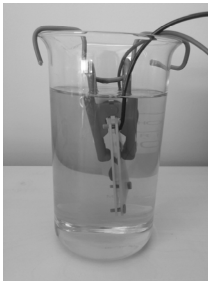
Fig.1. Diesel fuel sample with immersed electrodes
