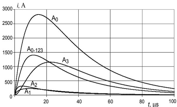
Fig. 7. The same currents as in Fig. 6 computed using a circuit approach implemented in ATP-EMTP. A simple double-exponential approximation of the injected current is adopted
