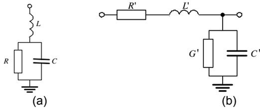
Fig.4. High-frequency models of (a) vertical and (b) horizontal ground electrodes
