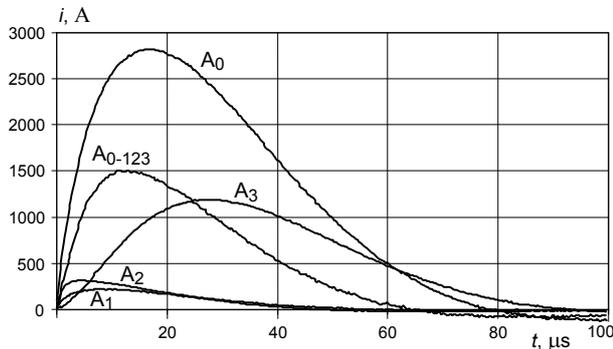
Fig. 6. Currents measured in test object; ( $A_0$  - current injected from the generator to air terminal of LPS,  $A_1$  and  $A_2$  - currents flowing into the LPS vertical ground electrodes,  $A_3$  - currents flowing into building electrical installation and cable neutral,  $A_{0-123}$  - calculated current  $A_{0-123} = A_0 - A_1 - A_2 - A_3$  flowing into the ground from the horizontal 20-m long flat bar connecting LPS with the cable termination box).
