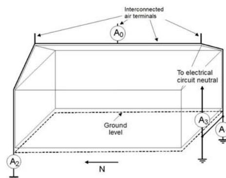
Fig. 2. Lightning protection system mounted on the test house with marked measurement points
