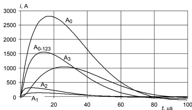
Fig. 8. The same currents as in Fig. 6 computed using a frequency-domain full-wave approach implemented in CDEGS. Accurate representation of the injected current created using point by point method is adopted.
