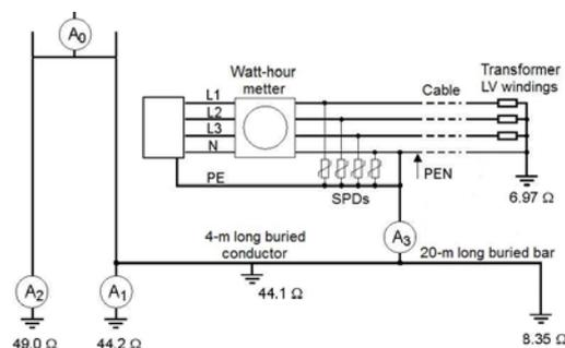
Fig. 3. Lightning protection system mounted on the test house with marked measurement points
