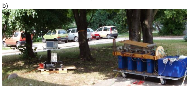
Fig. 4. Experimental setup (a) for SV measurement (G - high voltage generator, V - digital oscilloscope for SV record), b) photo taken during measurements
