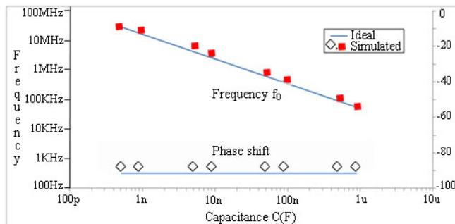
Fig.4. Corner frequency (Hz) and the corresponding phase shift (degree) of  $v_o/v_{in}$  versus the capacitance  $C(\text{F})$ , using a fixed bias current  $I_f$  value  $800 \mu\text{A}$ .
