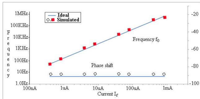
Fig.3. Corner frequency (Hz) and the corresponding phase shift (degree) of  $v_o/v_{in}$  versus the bias current  $I_f(\text{A})$ , using a fixed capacitance  $C$  of value  $0.08 \mu\text{F}$
