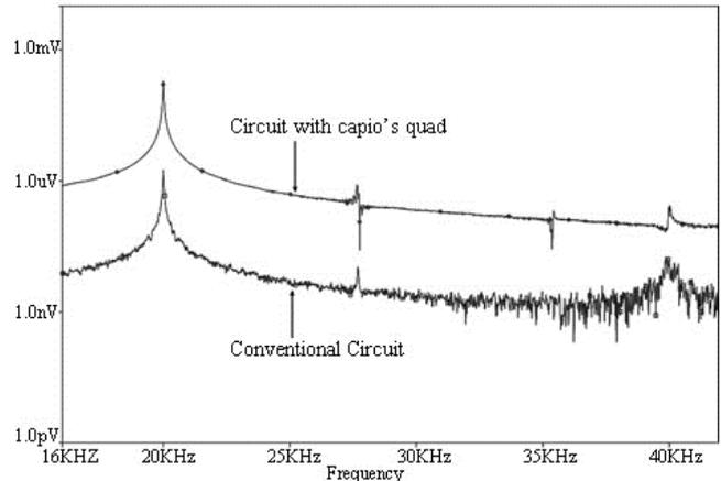
Fig.5. illustrates harmonic spectrums comparison of conventional circuit and circuit with Caprio's quad
