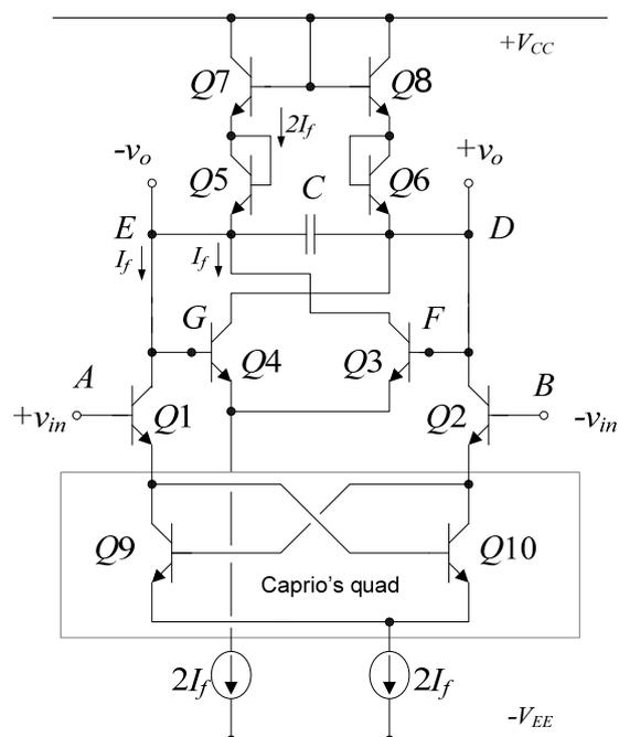
Fig.1. A fully-balanced current-tunable integrator with Caprio's quad
