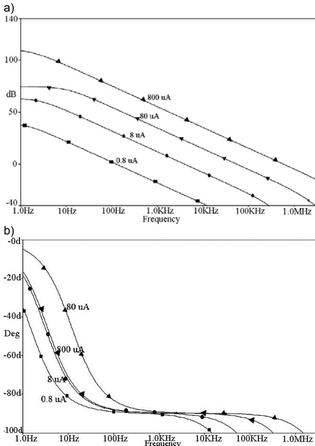
Fig.2. Magnitude (dB) and phase shift (degree) of  $v_o/v_{in}$  versus frequency (Hz) using the capacitance  $C = 0.08 \mu\text{F}$  and current  $I_f = 0.8 \mu\text{A}$ ,  $8 \mu\text{A}$ ,  $80 \mu\text{A}$ , and  $800 \mu\text{A}$
