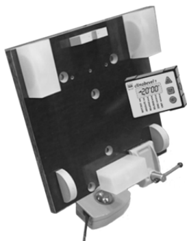
Fig.5. For the accuracy of the measurements a hip Phantom, composed of the three desired landmarks, was used and checked with the protractor Tesa Clino Bevel 1.
