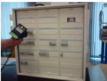
Fig. 4 Testing the immunity of the KNX model to electrostatic discharges
