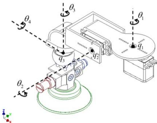
Fig.4. Scheme of robot leg with marked degrees of freedom
