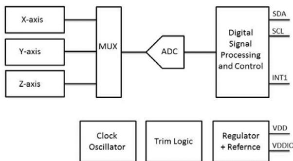
Fig.5. Sensor MAG 3110 - block diagram
