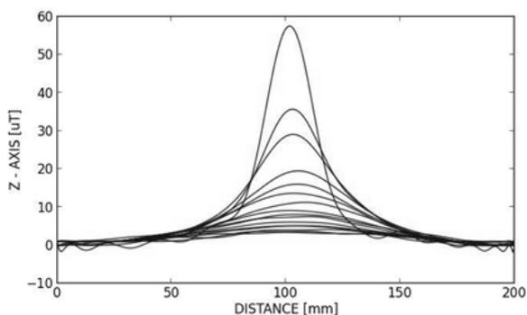
Fig.7. Result of rebars detection - measurements with sensor placed at the height of 10 to 100 mm
