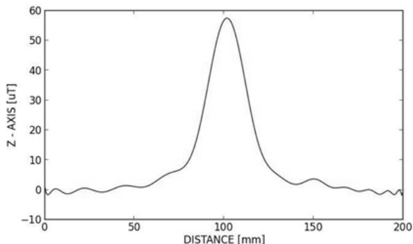
Fig.6. Result of rebars detection - one measurement with sensor placed at the height of 10 mm
