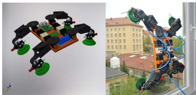
Fig.3. 3D visualization and photography of the Climbing Robot
