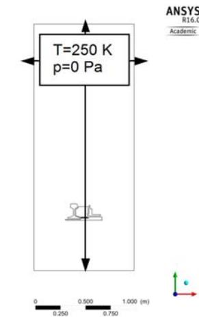
Fig. 4 The model of the railway turnout with the induction heater
