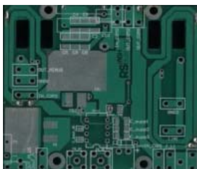
Fig. 9 The model of designed converter with PCB air choke.
