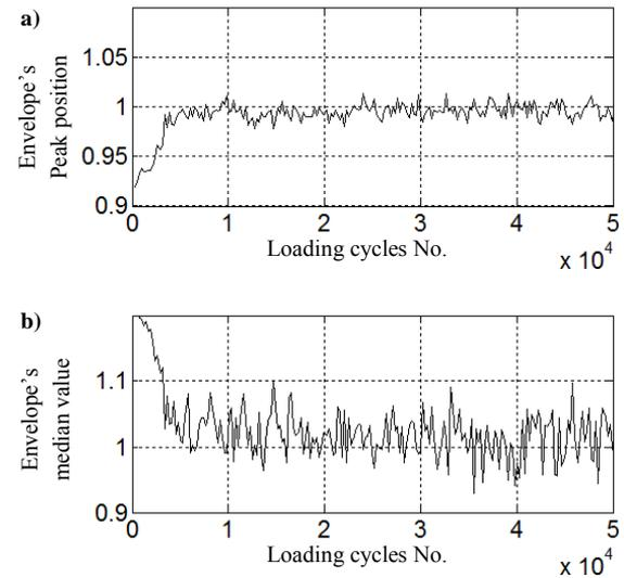
Fig. 6. Plots of BN envelope peak position (a) and median value (b) achieved at the beginning of the fatigue process; all distributions were normalized by the mean value of the parameters.
