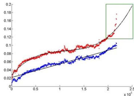
Fig. 7. The comparison of the maximum values from the sound region (blue line) and region of interest (red line). The rectangle marks the crack generation indication.
