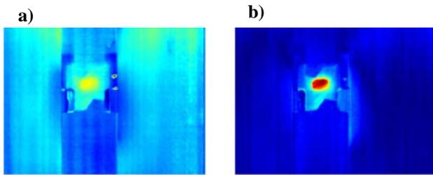
Fig. 9. The phase a) and amplitude b) images of the sample with crack generated in the load process
