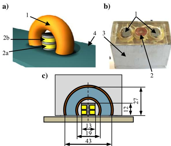
Fig. 2. Barkhausen noise transducer: three-dimensional view (a), photo (b) and cross-section view with dimensions (c) of the transducer; 1 – ferrite core, 2a- main pick-up coil, 2b – reference pick-up coil, 3 – shielding, 4 – examined sample.
