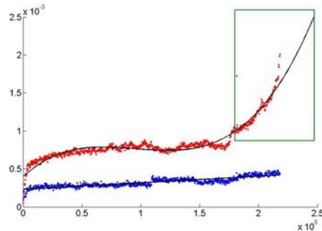
Fig. 8. The comparison of the standard deviation values from the sound region (blue line) and region of interest (red line). The rectangle marks the crack generation indication.
