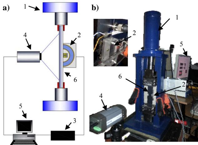
Fig. 1. Measuring system: a) schematic diagram, b) photo; 1 – fatigue stress machine, 2 – electromagnetic transducer, 3 – electromagnetic excitation and pick-up subsystem, 4 – Infrared camera, 5 – PC controlling and acquisition computer, 6 – steel sample.
