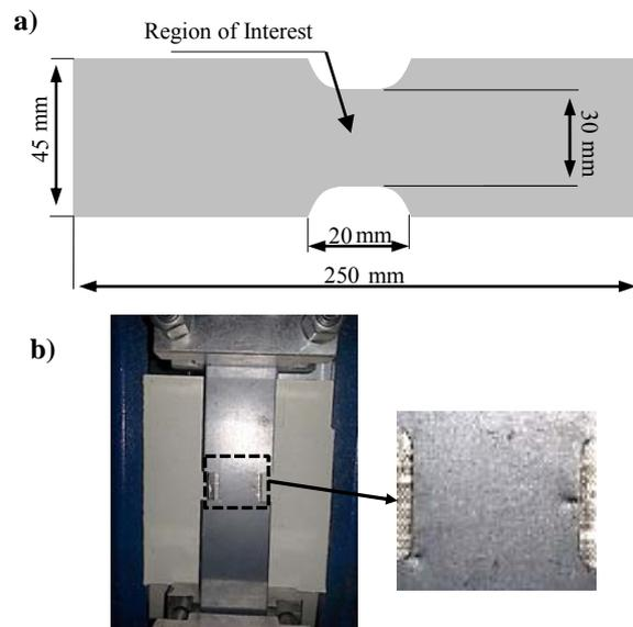
Fig. 3. View of fatigue loaded steel samples: a) draw with the shape and size of the samples, b) photo of the sample under fatigue test with enlargement of depicted (by black rectangle) region of interest.
