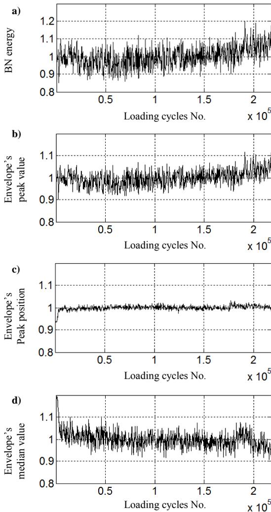
Fig. 5. Selected results obtained using Barkhausen noise method: a) BN signal's energy, b) envelope's peak value, c) envelope peak position, d) envelope's median value; all distributions were normalized by the mean value of the parameters.
