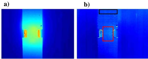
Fig. 4. Exemplary raw thermogram (a) and thermogram after normalization (b) with depicted sound region (black rectangle) and region of interest (red rectangle).
