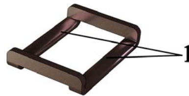
Fig. 4. 3D model of the one characteristic formed coil.
