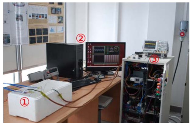
Fig.2. Test stand for measuring the electric response of the tape: 1 – HTS 2G tape in LN_2 bath, 2 – data acquisition, 3 – computer controlled supplying system
