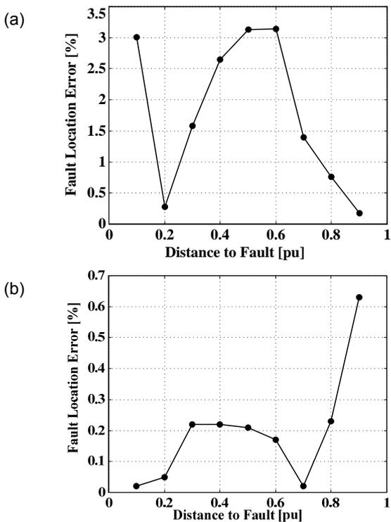
Fig. 7. Errors for locating broken conductor failure occurring: (a) in front of a-E fault, (b) behind a-E fault
