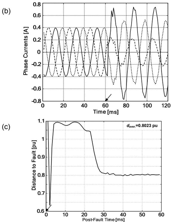
Fig. 6. Example of fault location – open conductor failure behind a-E fault,  $R_F=10 \Omega$ ,  $d=0.8$  p.u.: (a) secondary phase voltages, (b) secondary phase currents, (c) distance to fault
