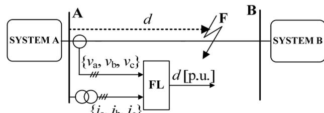
Fig. 1. Principle of one-end fault location
