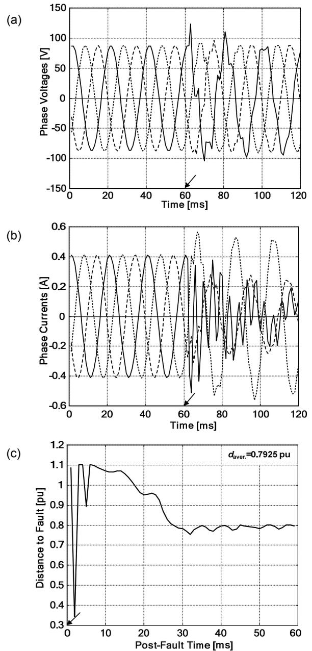
Fig. 5. Example of fault location – open conductor failure in front of a-E fault,  $R_F = 10 \Omega$ ,  $d = 0.8$  p.u.: (a) secondary phase voltages, (b) secondary phase currents, (c) distance to fault
