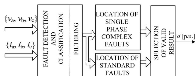
Fig. 3. Overall structure for locating typical and complex faults on power line
