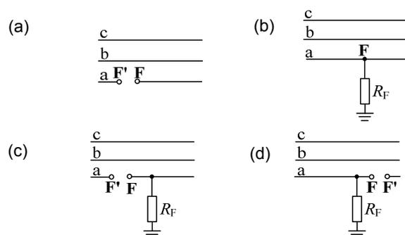
Fig. 2. Models of different faults: (a) open conductor failure alone (b) single phase-to-earth fault alone, (c) open conductor failure in front of earth fault, (d) open conductor failure behind earth fault
