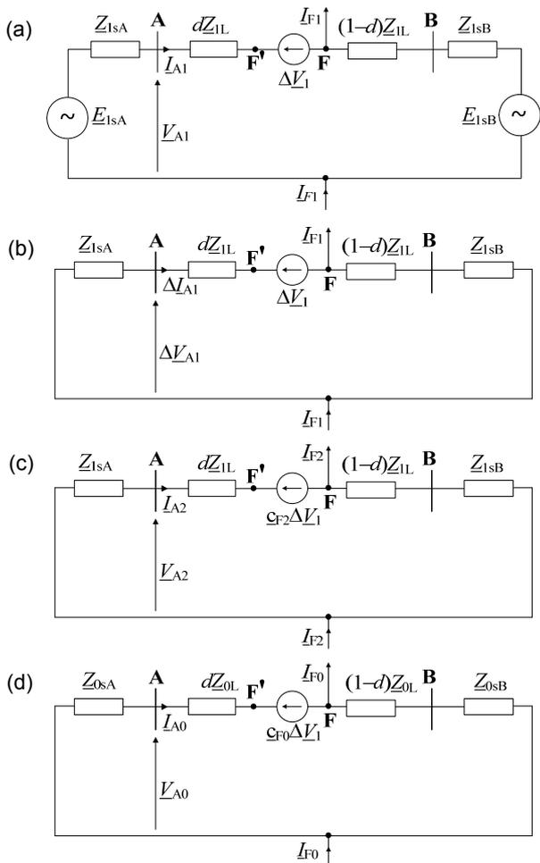
Fig. 4. The case of open conductor failure in front of earth fault – equivalent circuit diagrams of the transmission network for: (a) positive-sequence, (b) incremental positive-sequence, (c) negative-sequence, (d) zero-sequence
