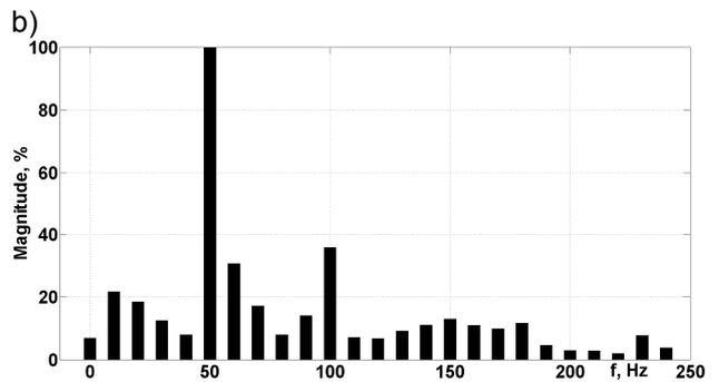
Fig.2. Harmonic content of the input (a) and output signal (b).
