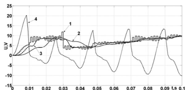
Fig.5. 1-OCF output signal, 2-HF output signal, 3-output signal of the HF with the shortened Hamming window, 4-fault signal which is proportional to the CT secondary current.
