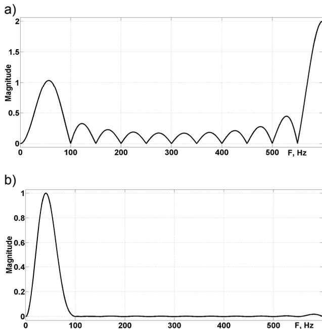
Fig.4. Frequency response: OCF (a), OCF with Hamming window (b)
