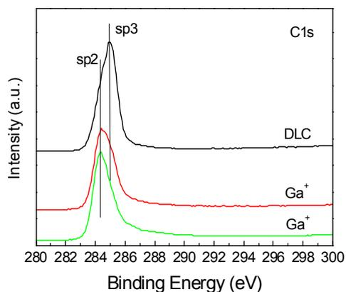
Fig.2. C1s spectra for unimplanted and  $Ga^+$  implanted samples with  $D_1 = 3 \cdot 10^{14} cm^{-2}$  and  $D_2 = 3 \cdot 10^{15} cm^{-2}$
