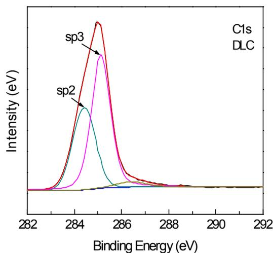
Fig.3. Deconvoluted C1s spectrum for unimplanted samples
