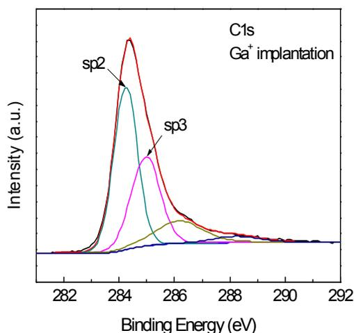
Fig.4. Deconvoluted C1s spectrum for  $Ga^+$  implanted samples with a fluence  $D_2 = 3 \cdot 10^{15} cm^{-2}$
