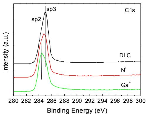
Fig.1. C1s spectra for unimplanted and  $N^+$  and  $Ga^+$  implanted samples with a fluence  $D_1 = 3 \cdot 10^{14} cm^{-2}$
