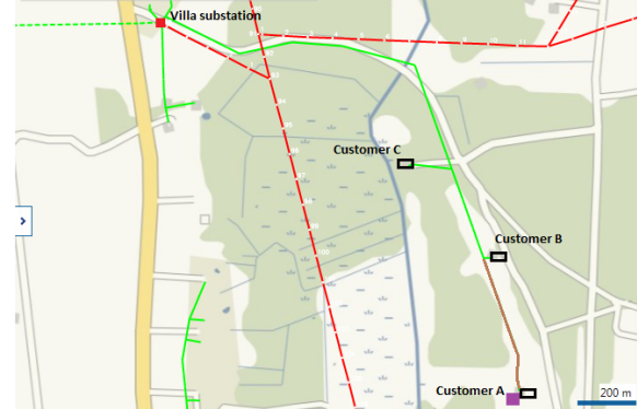
Fig. 1 Off-grid alternative for customer A (Villa F2)
