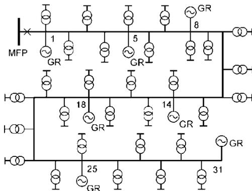
Fig. 1. The structure of the distribution medium voltage network together with the possible locations of the additional power sources (the figure does not reflect the network's branches)
