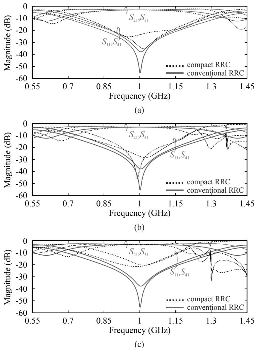
Fig. 4. S-parameters for selected design solutions with layout areas of: (a) 841 mm<sup>2</sup>, (b) 534 mm<sup>2</sup>, and (c) 353 mm<sup>2</sup>. Characteristics of a conventional RRC have been added for comparison purposes
