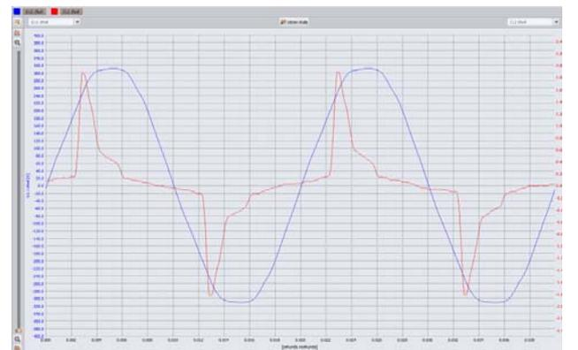
Fig.4. Voltage (blue/sinusoidal) and current (red/distorted signal) waveforms of 6 energy-saving bulbs studied together
