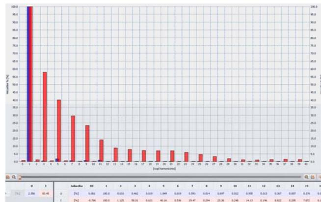
Fig.3. List of the power parameters of the PQM-700 analyser – the spectrum of current harmonics of 6 energy saving lamps working together
