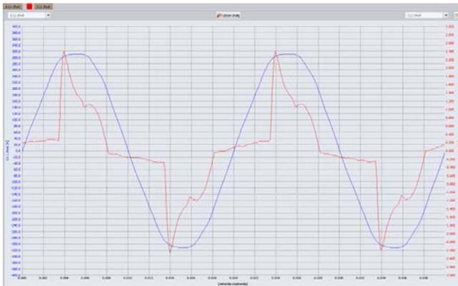
Fig.5. Voltage (blue/ sinusoidal) and current (red/ distorted signal) waveforms of two desktops working together
