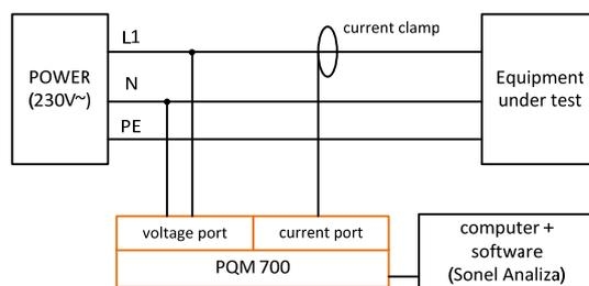
Fig.2. Block diagram for the measurement of power parameters
