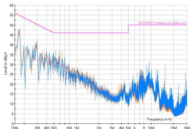
Fig.7. The measured values of conducted disturbances in the power supply circuit of 6 energy-saving lamps, range 150kHz-30MHz, AV detector, the orange line marks measurement in phase L1, the blue line – measurement in N, limit according to EN55022
