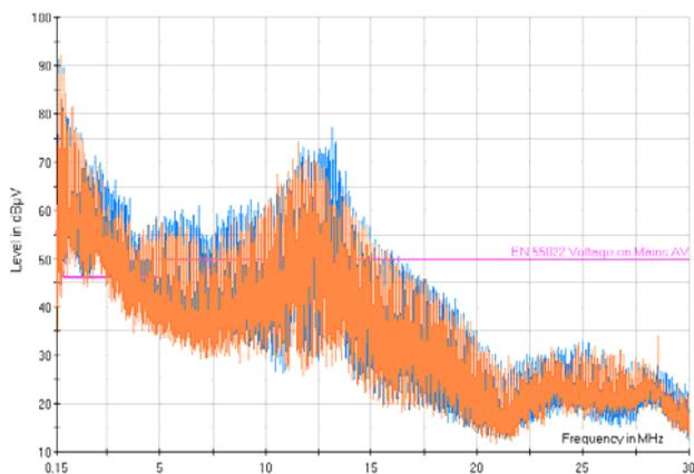
Fig.8. The measured values conducted disturbances in the power supply circuit of two desktop computers, 150kHz-30MHz, AV detector, the orange line marks measurement in phase L1, the blue line – measurement in N
