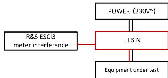
Fig.6. The block system for measuring disorders with line impedance stabilization network
