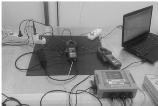
Fig.1. Photos from the study of power quality, a view of the PQM700 meter
