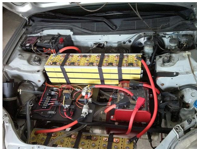
Fig.2. An example of improper placement of electric propulsion system elements [11]
