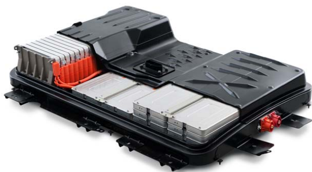
Fig.4. Structure of the battery box of a Nissan Leaf vehicle [7]
