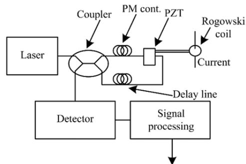
Fig. 5. Basic scheme of FOCS using Differentiating Sagnac Interferometer.
