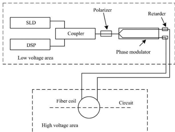
Fig. 3. Basic scheme of Sagnac fiber optic current sensor
