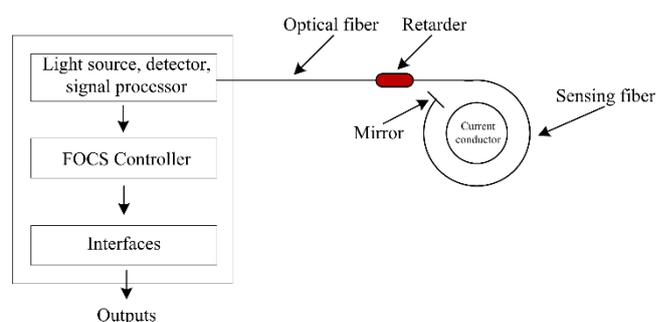
Fig. 2. Principle of the fiber-optic current sensor FOCS
