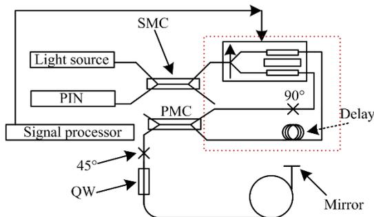
Fig. 6. Basic scheme of a novel fiber-optic current sensor.
