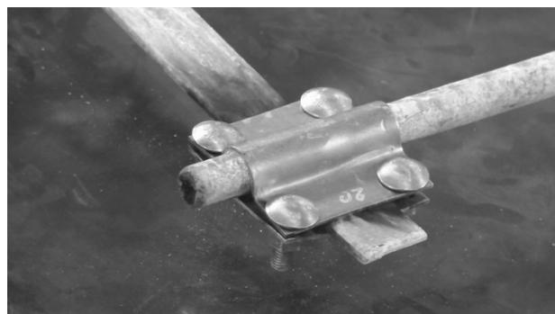
Fig.10 Cross connector assembled after the test with 100 kA current and shape 10/350  $\mu$ s
