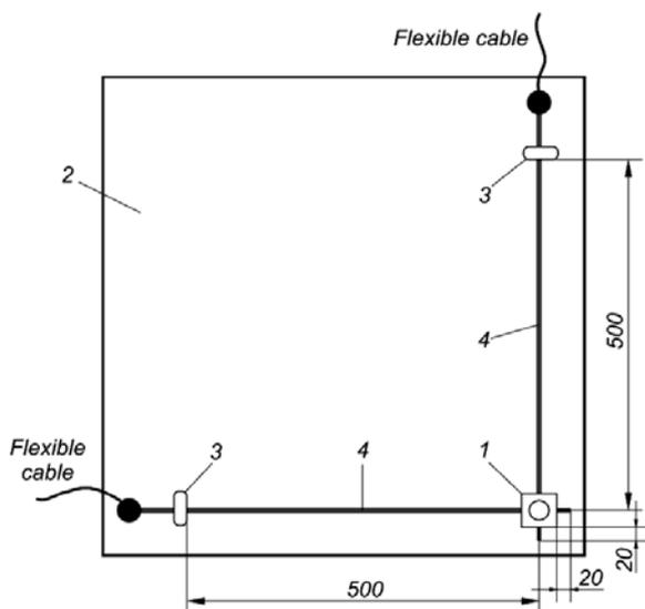
Fig. 3 The way to connect the given sample according to the PN-EN 62561-1:2012 [2] standard where: 1-Cross connection component, 2-Plate made of insulating material, 3-Rigid fastener, 4-Conductor and/or metal installation
