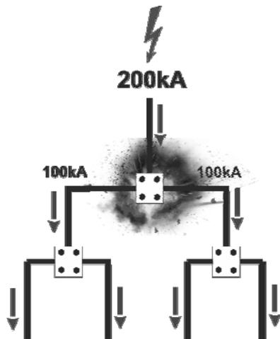
Fig.11 Lightning connection component explosion problem in EX zones because divergences in standards
