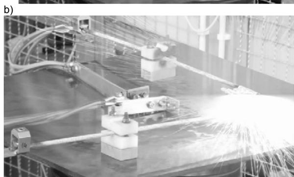
Fig. 7 Through galvanised connector before the test (a) and during the test (b) with 100 kA current and shape 10/350  $\mu$ s
