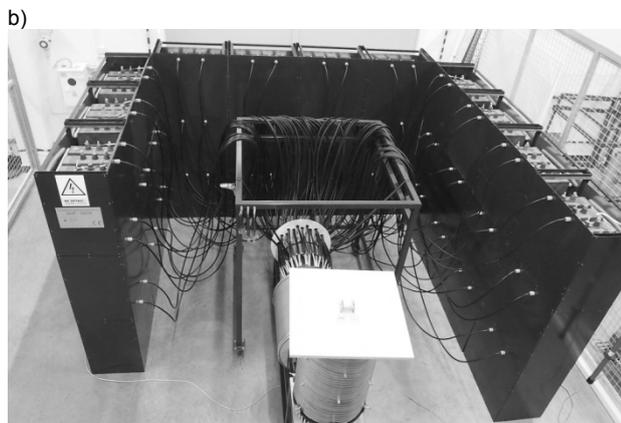
Fig.2 Generator of current surges: a) diagram of measurement system, b) generator view
