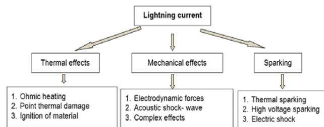
Fig. 1 Consequences of lightning current [1]
