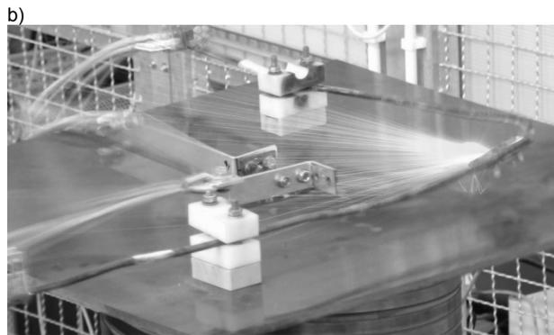
Fig.8 Through copper connector before the test (a) and during the test (b) with 100 kA current and shape 10/350  $\mu$ s
