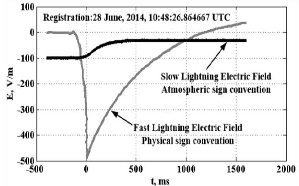
Fig.6. Registration of the lightning electric field selected for the computation of the calibration coefficient
