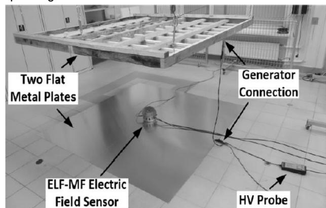
Fig.7. Measurement of the calibration coefficient at the high voltage laboratory
