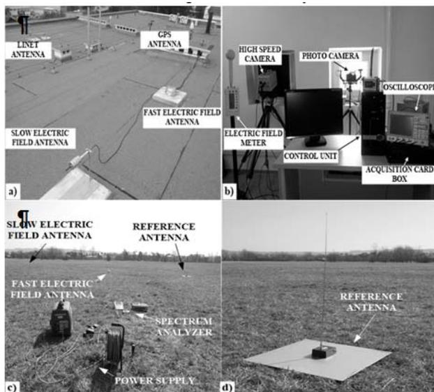
Fig.2. Measurement setup configurations. a,b) the first measurement point situated at the roof of Rzeszow University of Technology building; c,d) the setup located at the flat terrain
