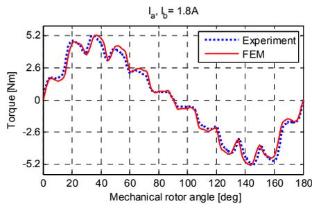
Fig.8. Static torque values – prototype B
