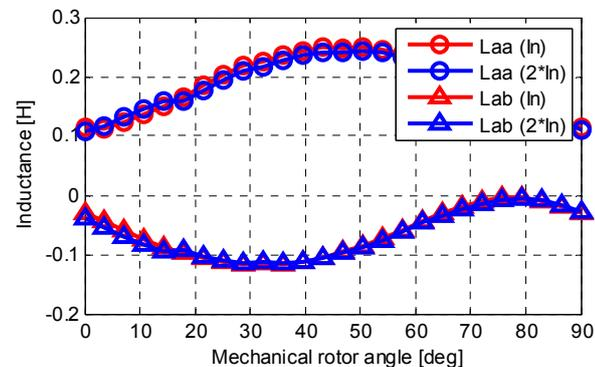
Fig.11. Self and mutual inductances; A (top) and B (bottom) - measurement results
