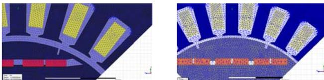
Fig.3. FE-meshes. Prototype A (left) and Prototype B (right)
