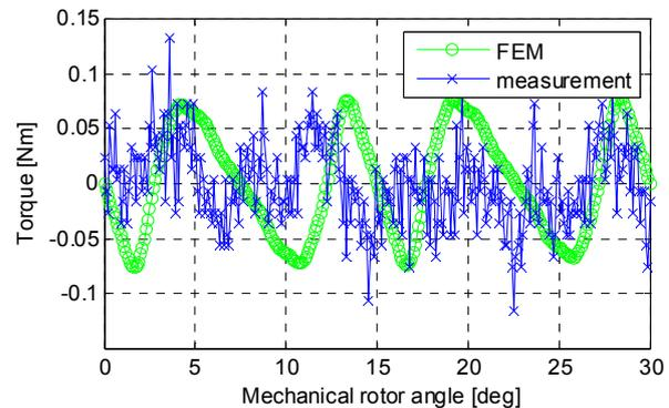
Fig.12. Cogging torque verification (prototype B)
