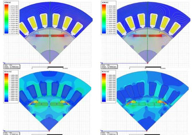
Fig.4. Prototype A – no load (left) and rated operation results
