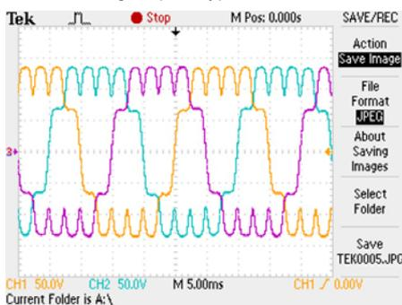
Fig.10. Induced voltage – prototype B
