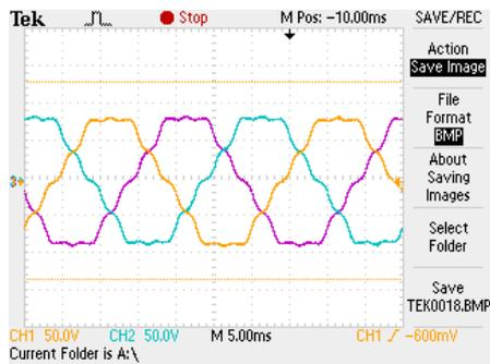
Fig.9. Induced voltage – prototype A
