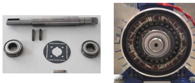
Fig. 1. Components of the IPMSM (left) and the opened housing (right)
