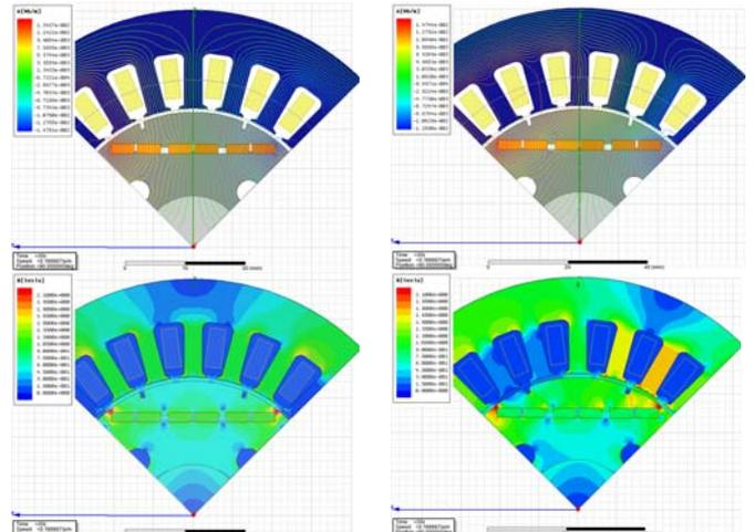
Fig.5. Prototype B – no load (left) and rated operation results
