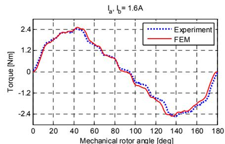
Fig.7. Static torque values – prototype A
