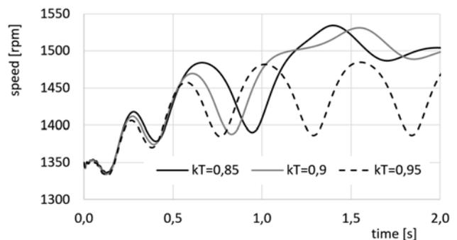
Fig.8. Example of successful and unsuccessful synchronization of four pole LSPMSM, rated load torque ratio  $kT=var$ , fan characteristic of the load torque, voltage drop during motor start-up  $\Delta u=20\%$ , top squirrel cage material bronze B8 type
