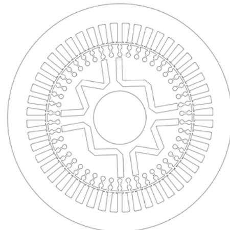
Fig.1. Cross-section of the 160 kW 2p=4 LSPMSM model
