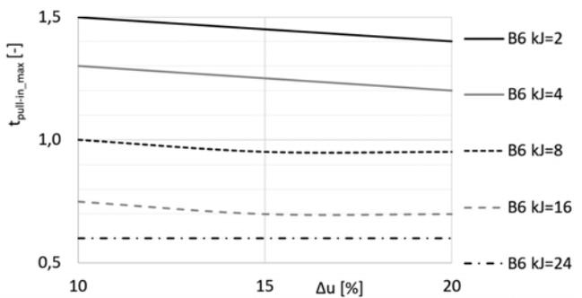
Fig.7. Influence of voltage drop during motor start-up  $\Delta u$  on the LSPMSM maximum pull-in torque  $t_{pull-in_{max}}$ , drive system moment of inertia  $kJ=var$ , top squirrel-cage material bronze B6 type
