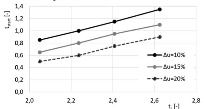
Fig.2. Influence of the LSPMSM starting torque  $t_r$  and voltage drop during motor start-up  $\Delta u$  on the maximum load torque  $t_{start}$
