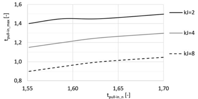
Fig.6. Influence of LSPMSM rated pull-in torque  $t_{pull-in_n}$  on the maximum pull-in torque  $t_{pull-in_{max}}$ , the drive system moment of inertia  $kJ=var$ , voltage drop during motor start-up  $\Delta u=15\%$
