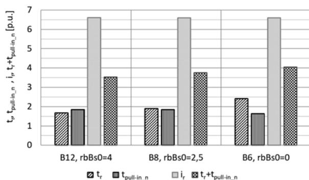
Fig.9. Influence of the top squirrel cage material (bronze type: B12  $\gamma=6,2$  MS/m, B8  $\gamma=7,5$  MS/m, B6  $\gamma=9,0$  MS/m) and bottom slots openings width  $rbBs0$  on the LSPMSM starting torque  $t_r$ , rated pull-in torque  $t_{pull-in,n}$  and sum of both torques, starting current  $i_r=const$
