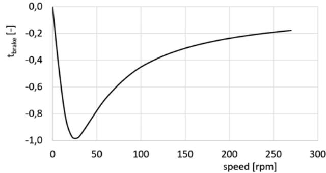
Fig.4. LSPMSM braking torque  $t_{brake}$  due to permanent magnets
