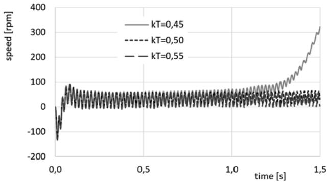
Fig.3. LSPMSM speed curves during start-up, voltage drop during motor start-up  $\Delta u=20\%$ , upper rotor squirrel cage material bronze B12, constant load torque, load torque value ratio  $kT=T_{load}/T_n=var$
