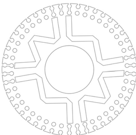
Fig.10. Cross section of double cage four pole LSPMSM without bottom slots openings
