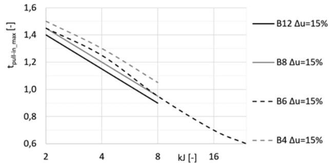
Fig.5. Influence of the drive system moment of inertia  $kJ$  on the LSPMSM maximum pull-in torque  $t_{pull-in_{max}}$ , top squirrel cage material bronze type: B12  $\gamma=6,2$  MS/m, B8  $\gamma=7,5$  MS/m, B6  $\gamma=9,0$  MS/m, voltage drop during motor start-up  $\Delta u=15\%$
