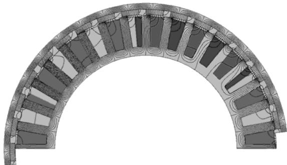
Fig.4. Magnetic field distribution for calculated nominal value of rotational torque
