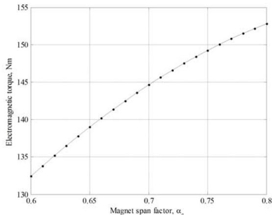
Fig.7. Dependence of mean electromagnetic torque value on magnet span for nominal current and quadrature-axis rotor position
