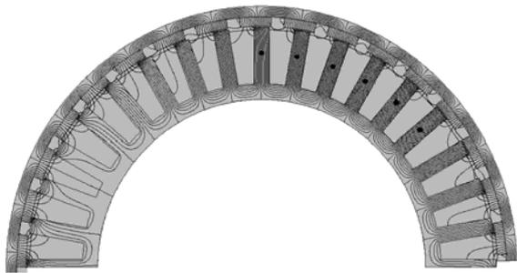
Fig.3. Magnetic field distribution created by magnets in the half of motor cross-section
