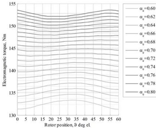
Fig.6. Instantaneous and mean values of electromagnetic torque in respect to rotor position for nominal current and quadrature-axis rotor position for different magnet span
