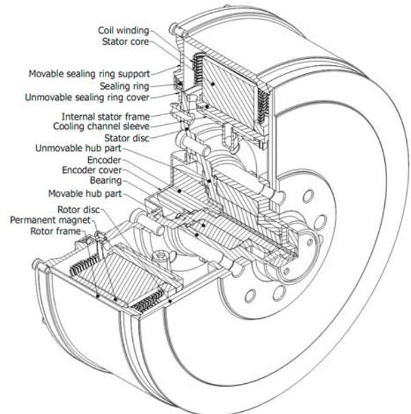
Fig.2. Main parts of the assembled PMSM
