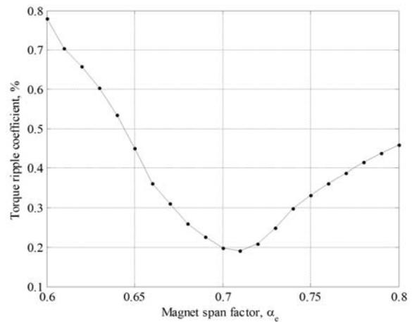
Fig.8. Dependence of torque ripples coefficient on magnet span for nominal current and quadrature-axis rotor position
