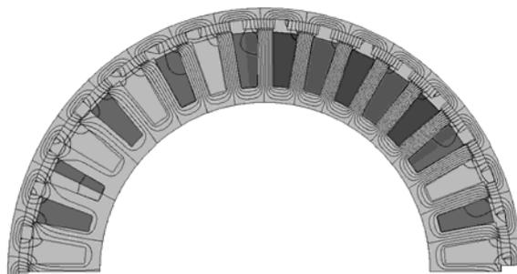
Fig.5. Magnetic field distribution for direct-axis synchronous inductance calculation for conforming stator and rotor fluxes
