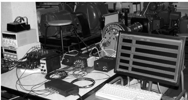
Fig.11. View of laboratory stand for vibration and induced voltage tests
