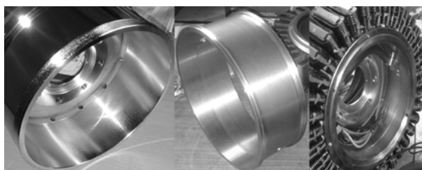
Fig.8. Stator frame, cooling channel ring, complete cooling channel with pipes
