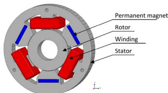
Fig.1. Construction of the HMB actuator
