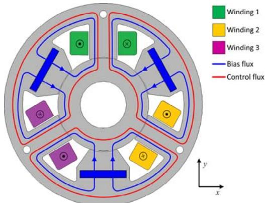
Fig.2. Paths of the magnetic flux in the HMB actuator
