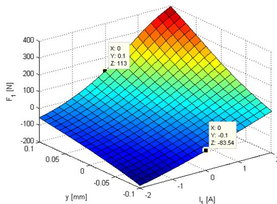
Fig.8. Magnetic force  $F_1$  in function of the current  $I_1$  and the rotor position  $y$
