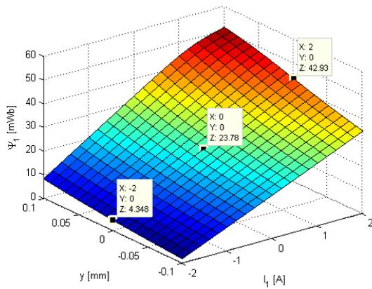
Fig.9. Flux linkage  $\Psi_1$  in function of the current  $I_1$  and rotor position  $y$
