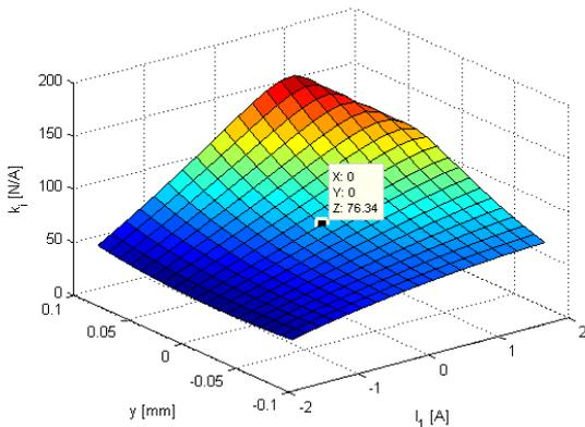
Fig.10. Current stiffness  $k_i$  in function of the control current  $I_1$  and rotor position  $y$
