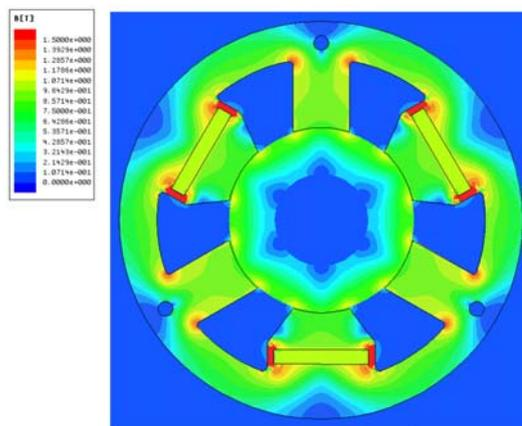
Fig.3. Magnetic flux density distribution in the HMB under central position of the rotor currents  $i_1 = i_2 = i_3 = 0A$
