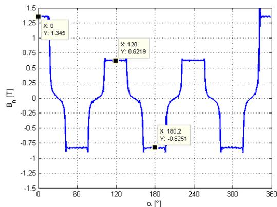
Fig.7. Normal (to the stator surface) component of the magnetic flux density in the air gap for central position of the rotor and currents  $I_1 = 2A$ ,  $I_2 = I_3 = 0A$
