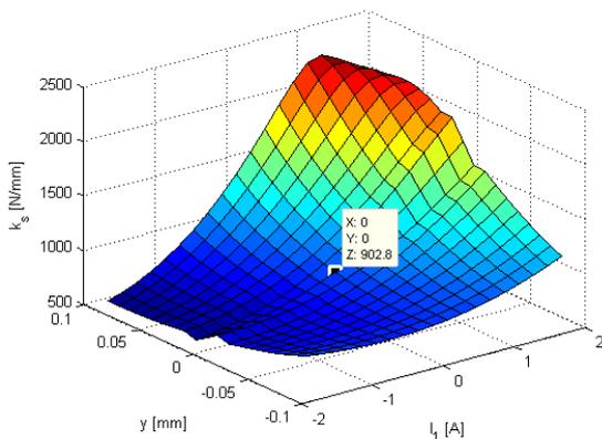
Fig.11. Position stiffness  $k_s$  in function of the control current  $I_1$  and rotor position  $y$
