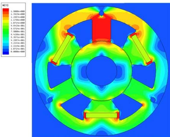
Fig.6. Flux density distribution in the HMB for central position of the rotor and currents  $I_1 = 2A$ ,  $I_2 = I_3 = 0A$
