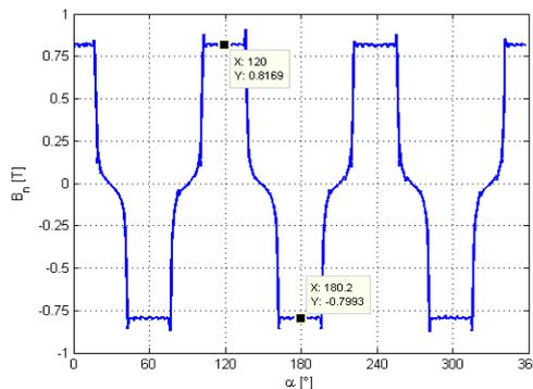
Fig.4. Normal component (to the stator surface) of flux density, in the air gap, for the central position of the rotor and currents.  $i_1 = i_2 = i_3 = 0A$
