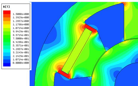
Fig. 5. The zoom of the magnetic flux distribution in the area of permanent magnet pole
