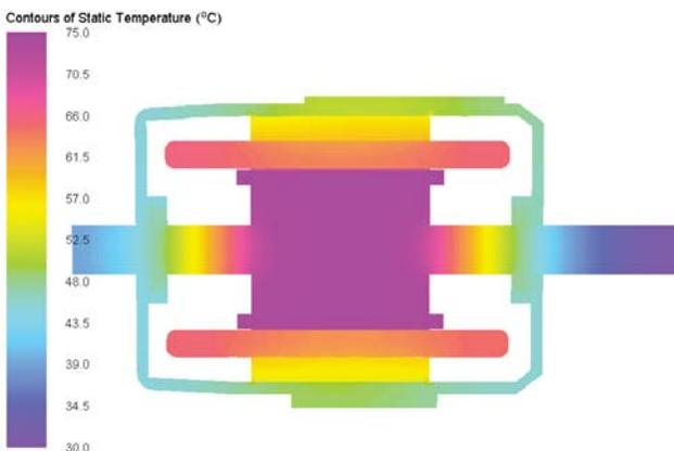
Fig. 5. The temperature distribution in the axial section of the machine
