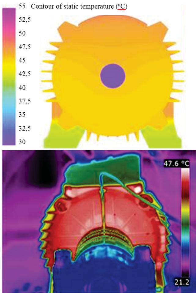
Fig. 7. Comparison of the temperature distribution on the frontal surface of the motor
