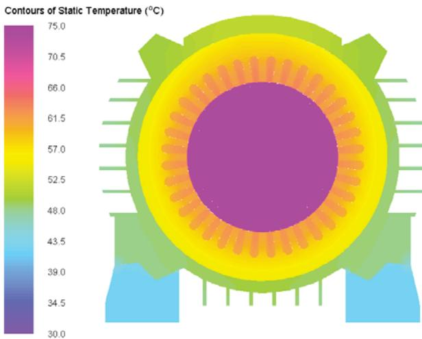
Fig. 4. The temperature distribution in the cross section of the machine
