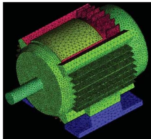
Fig. 3. View of the mesh on the surface of the motor
