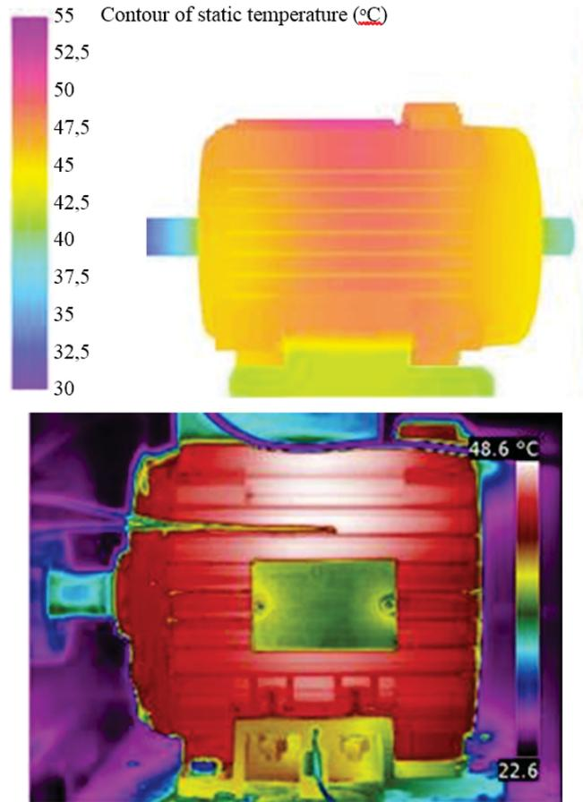
Fig. 6. Comparison of the temperature distribution on the side surface of the motor
