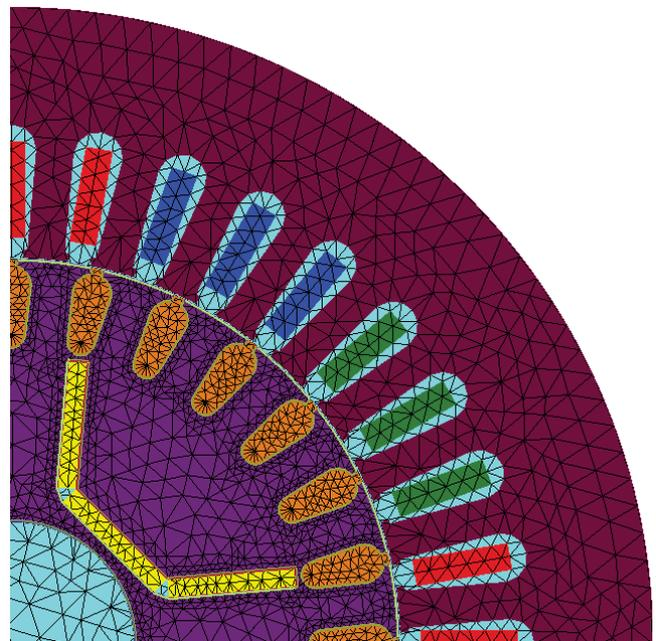
Fig. 1. A quarter of the mesh used in Finite Element Analysis
