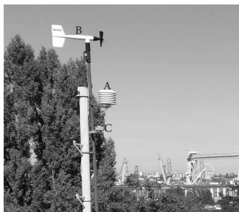
Fig. 1 Sensors of the weather station situated on the mast of the building of Gdynia Maritime University (A -termohigrometer, B - the wind-gauge, C - the sensor of power density of the solar radiation)
