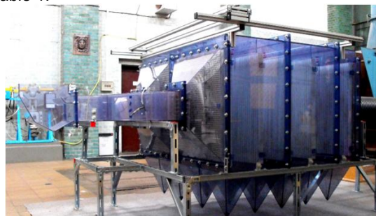
Fig. 1. Physical model of studied ESP
