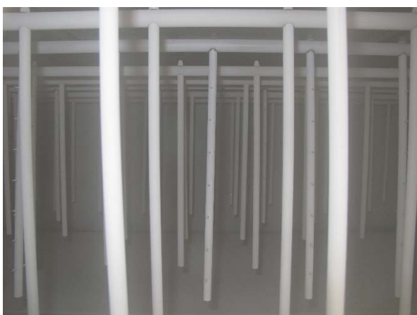
Fig. 3. Electrodes of experimental precharger/agglomerator (covered by fly-ash)
