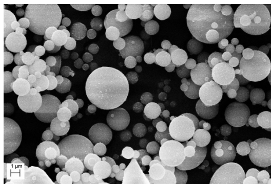
Fig. 5. SEM micrograph of fly ash particles used in the experiments (SEM Zeiss EVO 40).
